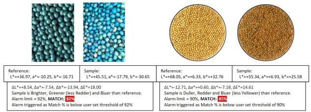
Sensegood Spectrophotometer for color measurement and quality - consistency control in color coated and natural seeds
